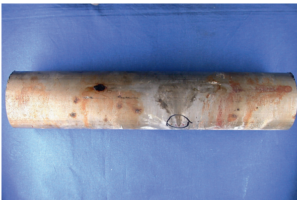
Fig. 3: Another location on the outer surface of the pipe with coatings and places of damage (circle) \approx 1:3
