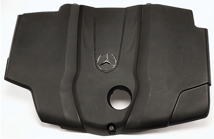
Figure 1.13 Mercedes-Benz engine cover for in-line four-cylinder diesel engine OM651 molded using a polyamide 6 reinforced with glass fibers and iM1 6K glass bubbles PA6 achieving a weight reduction of 20% versus the previous polyamide reinforced with glass fibers only (Courtesy of 3M Company)
