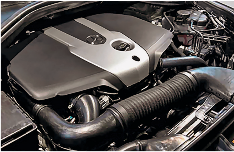
Figure 1.14 Mercedes-Benz engine cover assembled on OM651 engine (Courtesy of 3M Company)
