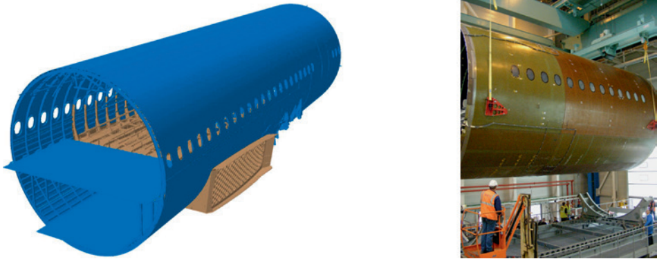
Figure 4.16 Carbon fiber reinforced composite fuselage structures [Courtesy: Airbus Operations GmbH]
