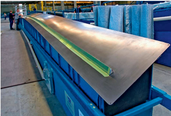
Figure 6.3 Steel tooling for the manufacture of rotor blades [Courtesy: Premium Aerotec GmbH]
