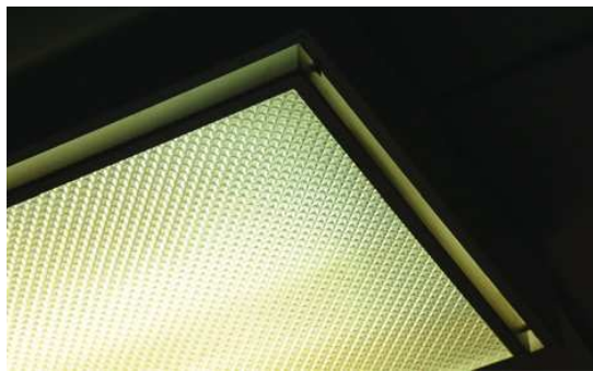
Figure 2.28 PMMA is much used by the lighting industry, e.g. as a screen for fluorescent tubes.
