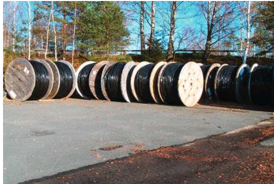
Figure 2.8 Cable jacketing. LDPE is used in the extrusion of jacketing for high voltage cables
