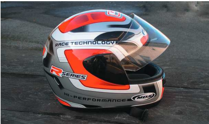
Figure 3.29 Polycarbonate is both incredibly impact resistant and suitable for painting, making it an excellent material for motorcycle helmets. The visor is also produced in polycarbonate.
