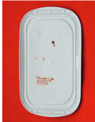
Figure 29.23 Here there are brown greasy oil stains on a white plastic cap.
