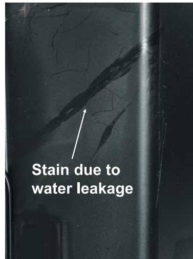
Figure 29.24 Here there is a diagonal mark on the surface that was formed when plastic melt came in contact with water in the cavity.
