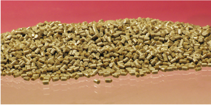
Figure 1.2 Shape of PEK granules
