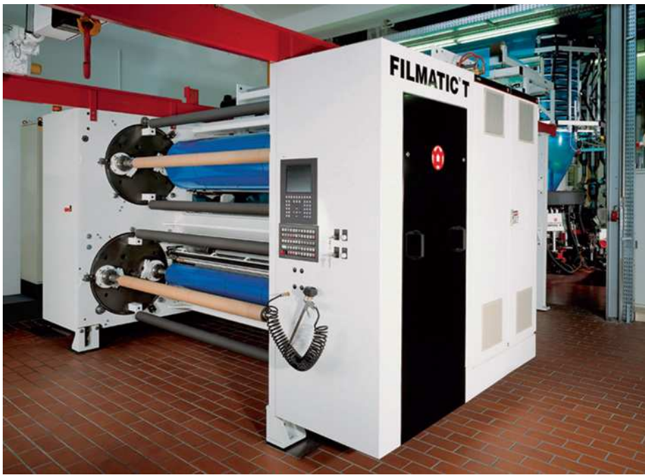
Figure 4.20 A dual-station turret winder ( Windmoeller & Hoelscher )
