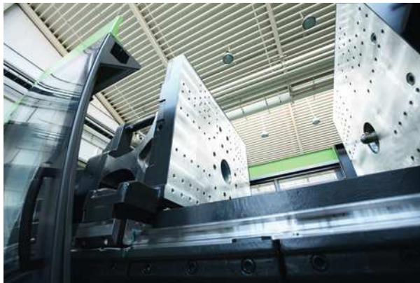
Figure 13.4 Tie-barless clamping unit detail; source: Helmut Roegele
