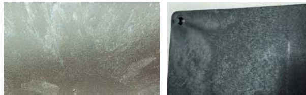
Figure 25.5 Examples of streaks caused by trapped air; source: Ascamm
