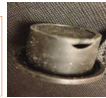
Figure 25.7 Weld lines between two flow fronts can cause air entrapments
