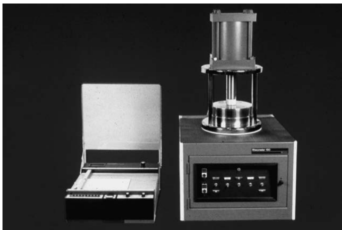
Figure 1.7 The Monsanto Model R100 Oscillating Disc Rheometer with a flat bed chart recorder. This curemeter revolutionized cure testing in the rubber industry and was the recipient of a Trilogy Award in 2000; Reprinted with permission from Alpha Technologies.
