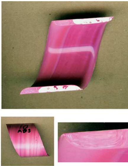
ABS segment at 10th L/D from 63.5 mm (2.5 in.) D., L/D = 21 , screw with a square-pitch flight ( 17.65^\circ helix angle)
