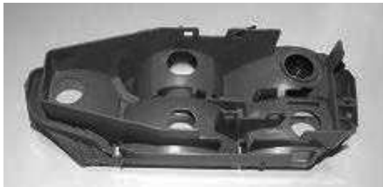
Detail of reflector from tail-lamp assembly showing part complexity
