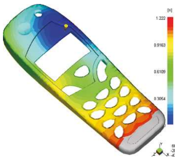
Figure 5.8 2½-D mold filling analysis output of fill pattern
