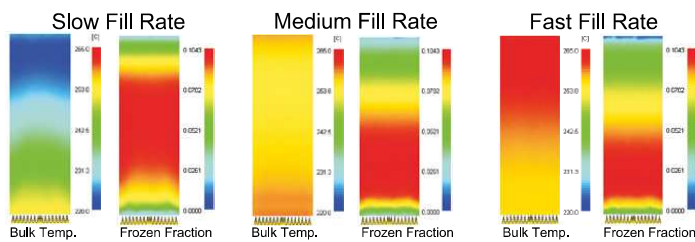
Figure 3.1 Effects of injection rate on bulk melt temperature and frozen material fraction as predicted by Moldflow's MPI
