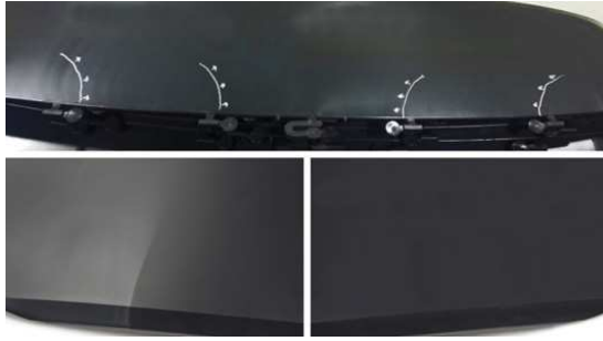
Figure 11.25 Automotive part where the left side was molded with a traditional fast-opening valve gate versus the right side that was molded using a profiled servo driven valve gate (Courtesy: HRSflow)
