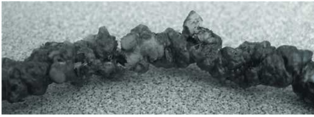
Figure 6.16 Unmelted plastic pellets in the purge as a result of moving too fast through the molding barrel
