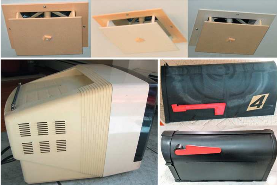
Figure 2.30 Long term yellowing and fading of plastics
