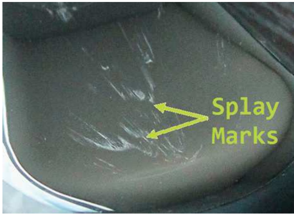
Figure 5.41 Splay due to moisture in the resin [9]
