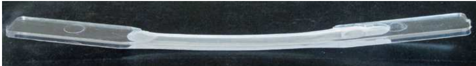
Figure 2.37 Stress relief with machining
