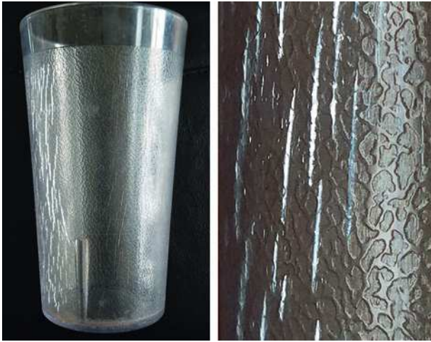
Figure 3.38 Stress crazing in a clear polystyrene tumbler
