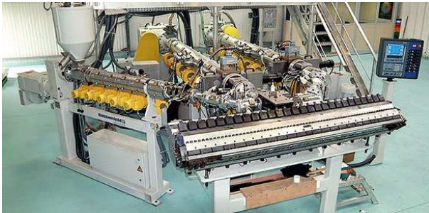
Figure 2.4 Coextrusion with three extruders, feed block, and coat hanger die, courtesy of Battenfeld
