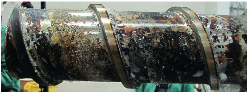
Figure 1.12 Photograph of a screw that had numerous shutdowns where the extruder was maintained at operating temperatures for an extended time. The extruder was purged prior to removing the screw, yet dark degraded resin covers most areas of the screw [1]
