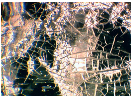
Figure 11, GF-UP sheet, transparent (M = 20, AL + DL). The cracks (hair cracks) in the sample surface developed after 5000 hours of weathering in a Xenon tester 1200 CPS. The crack depth is no deeper than about 35 \mu\text{m} . During recording, a low level of transmitted light has been combined with incident light.
