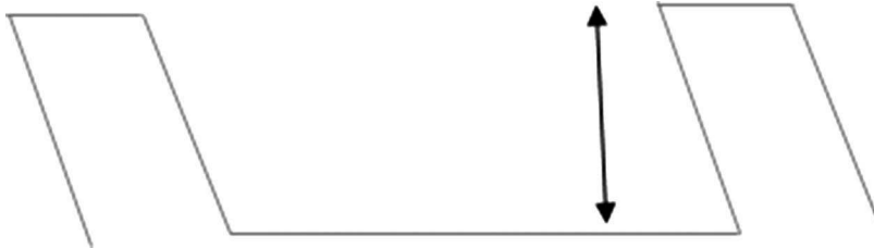
Figure 1.8 Measuring flight depth in feed section
